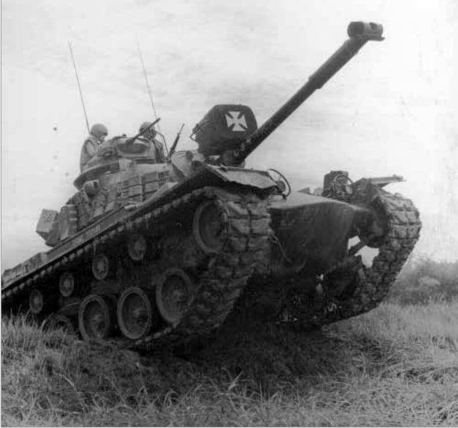
Dick Peksens writes: I found this photo online of one 3rd Platoon of Charlie Company (recognizable with the Maltese cross). Not sure when it was taken or if it was previously posted in SB. I like it because it shows the vulnerable underbelly of an M48 when traversing a dike. This is usually when the NVA would take a shot with an RPG to take advantage of the minimal 2 inches of steel....
