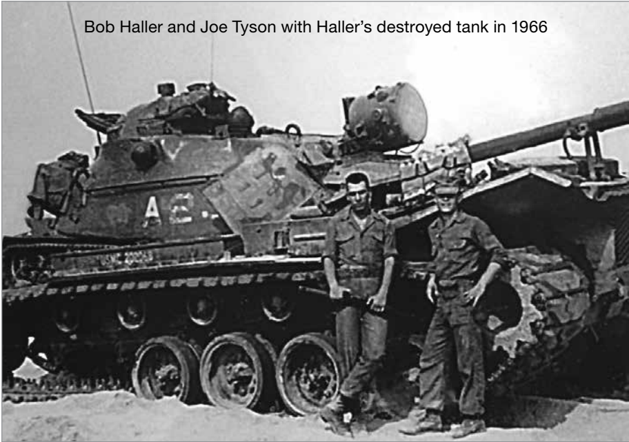
Dick Peksens writes: I found this photo online of one 3rd Platoon of Charlie Company (recognizable with the Maltese cross). Not sure when it was taken or if it was previously posted in SB. I like it because it shows the vulnerable underbelly of an M48 when traversing a dike. This is usually when the NVA would take a shot with an RPG to take advantage of the minimal 2 inches of steel....
